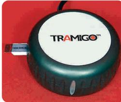
Use a flat instrument to gently push the SIM all the way in (2 mm past edge of case). If the SIM will push further than 2mm into the T21 you have missed the track, so remove the SIM and re-insert keeping the SIM sliding on the lower half of the slot.
