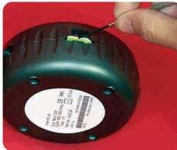
SIM installed with a removal tape showing.
