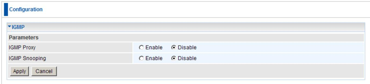
The screenshot shows a configuration window titled "Configuration" with a sub-section for "IGMP". Under "Parameters", there are two rows: "IGMP Proxy" and "IGMP Snooping". Each row has two radio buttons: "Enable" and "Disable". In both cases, the "Disable" radio button is selected. At the bottom of the configuration area, there are "Apply" and "Cancel" buttons.
