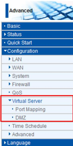
In TCP and UDP networks a port is a 16-bit number used to identify which application program (usually a server) incoming connections should be delivered to. Some ports have numbers that are pre-assigned to them by the IANA (the Internet Assigned Numbers Authority), and these are referred to as “well-known ports”. Servers follow the well-known port assignments so clients can locate them.
