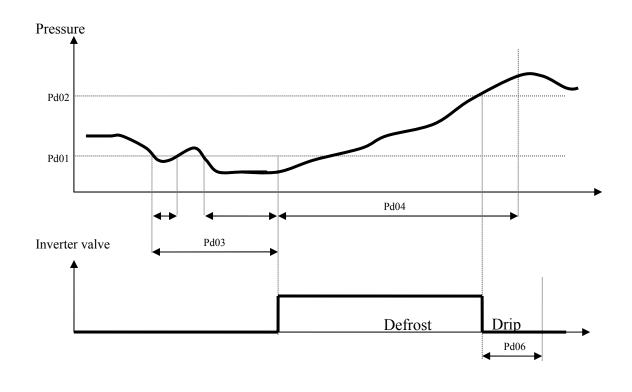
In order to avoid the immediate start of a defrosting cycle after all compressors have been stopped, a *Minimum circuit restart delay Pd07* is used. This provides at least a period of heat-pump operation before entering the defrosting cycle.
