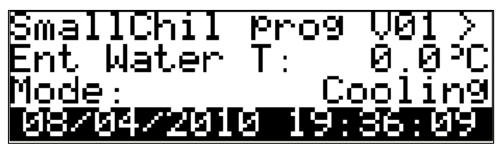
By pressing the RIGHT or LEFT buttons in this page, it is possible to display other information like circuit status, RTC, or all the configured sensors. In case of the inoperable status of the sensors, the value field of the corresponding sensor displays ---- if the sensor is enabled else displays .... if the sensor is disabled.
