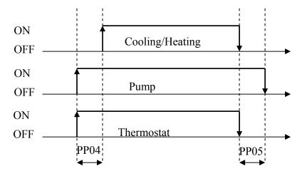
In a similar fashion, on a thermostat switch-off request, the compressor switches off, while the pump remains on for the duration of *PP05*.
