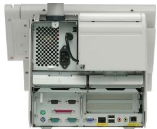
A look to the many interfaces and HDDs (opened rear cover)
