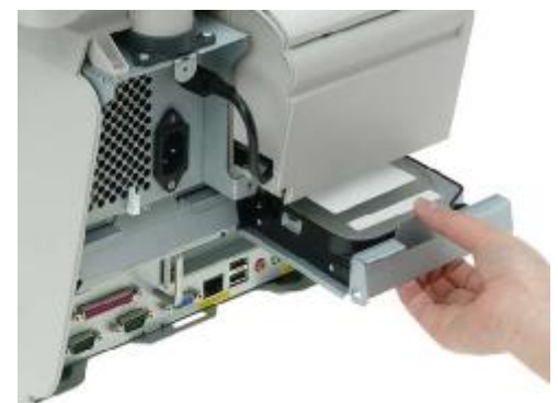
The HDDs are easy to reach and ensure protection of the important data via RAID Controller.
