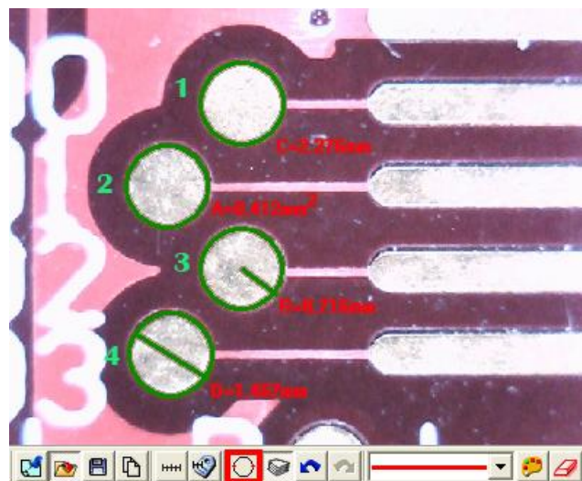
Fig 5-63 2 Points Circle Measurement
