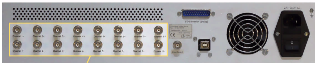
The 8 pairs of output lines are available on 16 BNC output connectors at the rear side of the device
