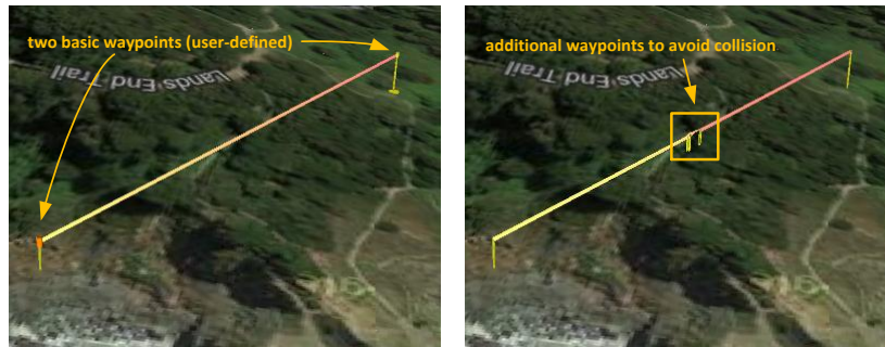
Figure 22. Additional waypoints inserted between the basic ones.
