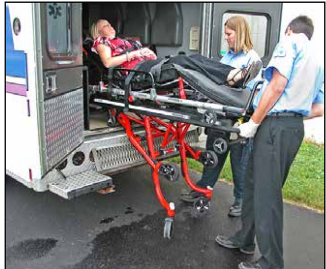
Figure 21 - After the Control-End Legs Unfold, Check the Indicator to Verify the Legs Have Locked
