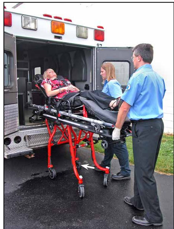
Figure 22 - Unloading the Transporter
