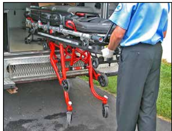
Figure 26 - One Operator Loading or Unloading
