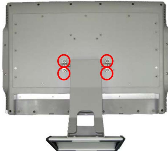
**Step 4** Assembly the hinge cover and fix the screws as marked on the back side of chassis (Use Screw C).
