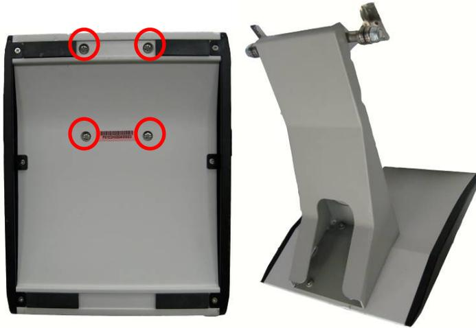
**Step 3** Fix the screws as marked on the back side of chassis (Use Screw B).
