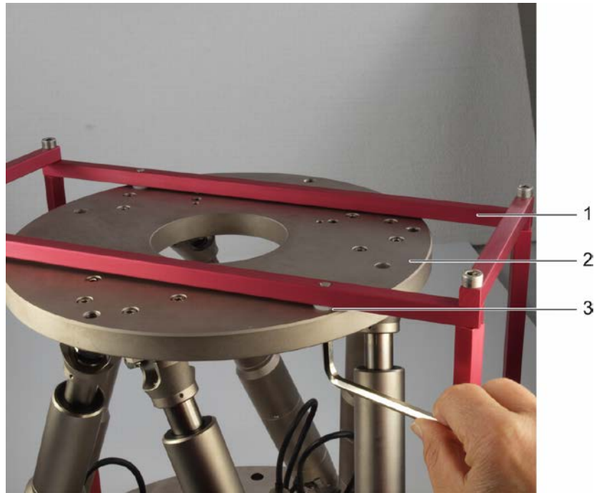
Figure 10: Transport lock on the moving platform
