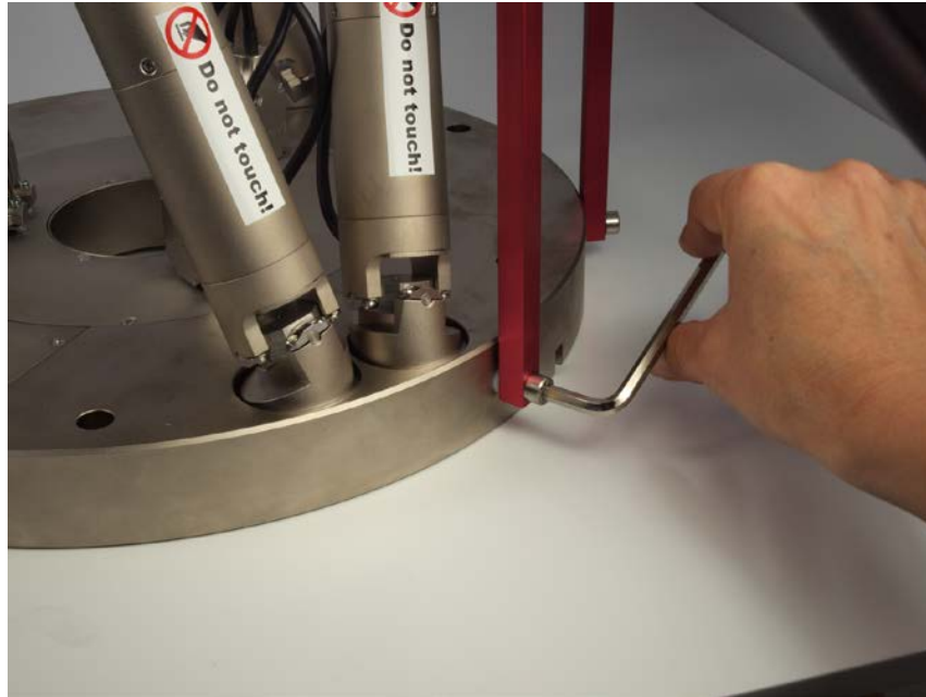
Figure 11: Transport lock on the base plate
