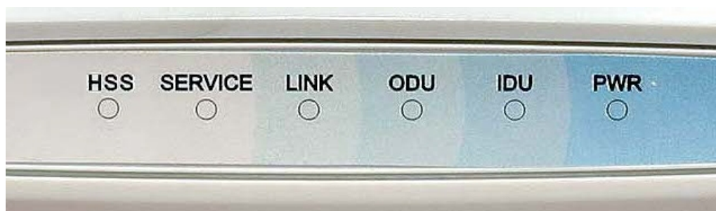
Figure 7: IDU-NetStream DT Front Panel LEDs
