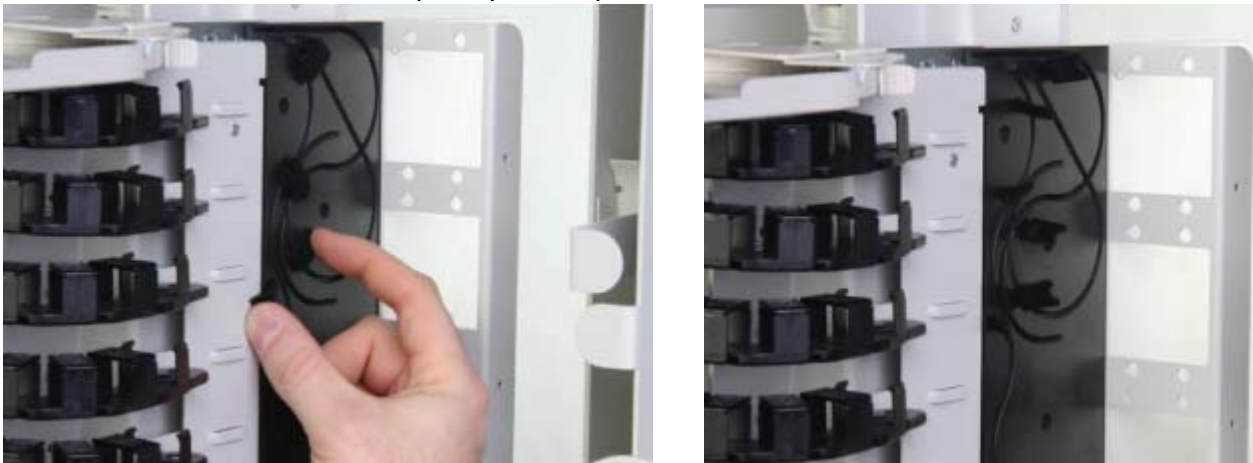
Figure 15 - Opening the hook-and-loop straps
