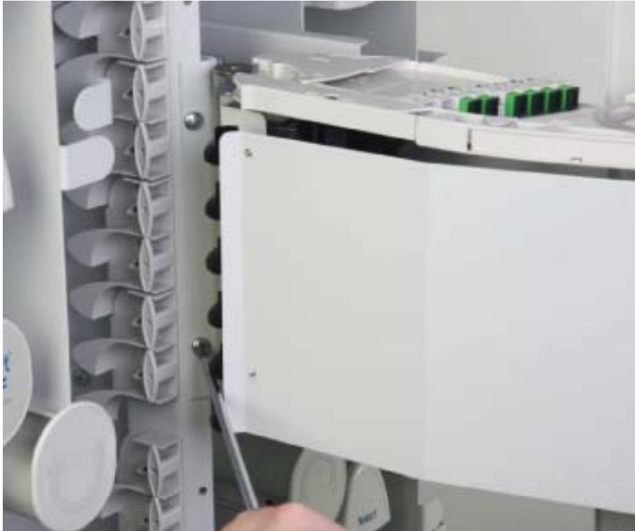
Figure 7 - Securing the Module
