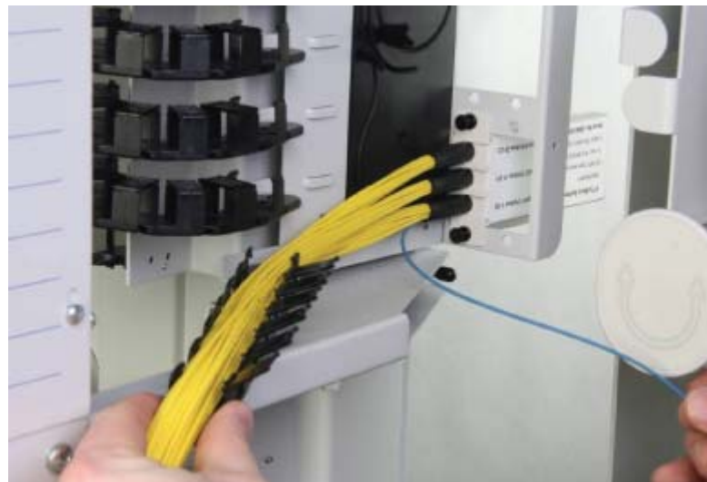
Figure 17 - Threading the Legs
