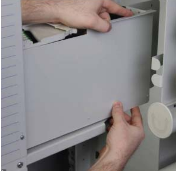
Figure 10 - Lifting off the Cover
