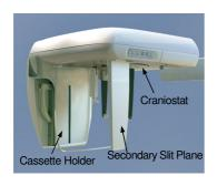
Hold the bottom of the cassette with one hand and the grip with the other. Push down the button and carefully slide the cassette into the holder until the rod goes inside. Then release the button.
