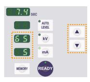
Press the kV key to display the tube voltage value. This value can be changed. Use the Up and Down keys to increase or decrease the value.
