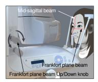
Keep the patient's Frankfort plane horizontal and align the beam with the patient's external auditory orifices by turning the Frankfort plane beam Up/Down knob. Then hold his head in place by lightly closing the temple stabilizers.
