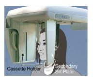
11. The cassette holder and secondary slit plate will move into their starting positions.
