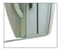
3. During image transmission the LED on the cassette will light up amber. After transmission is completed, it will change to green and start blinking. ("Transferring image!" will appear in the computer display, and after about 30 seconds the image will appear.)
