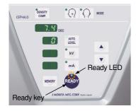
Press the Ready key on the arm operation panel or the patient frame to automatically move the arm to the patient entry position.
