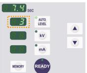
The current auto level value is shown on the left side of the Auto Level key. This value can be changed. Up and Down keys will also appear to the right; use these to change the settings.
