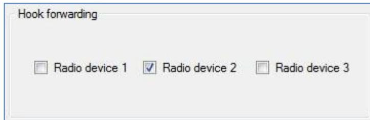
Figure 25: Selection of radio devices for hook forwarding
