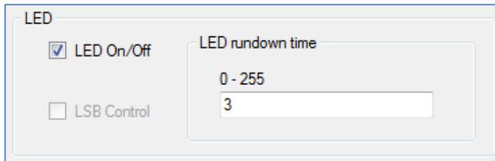
Figure 24: Settings for LEDs and LSB
