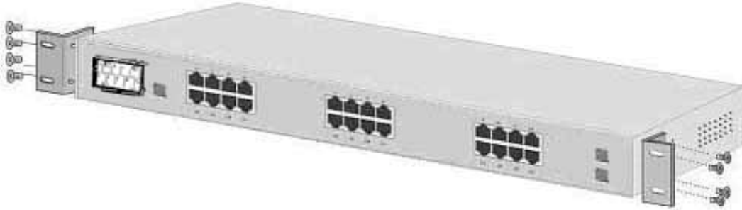
Figure 2-4. Attach mounting brackets with screws
