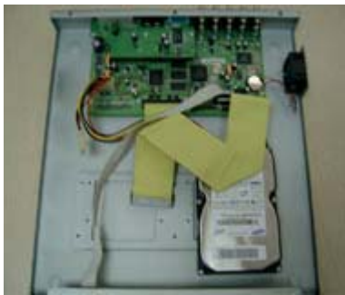
One HDD Installation
