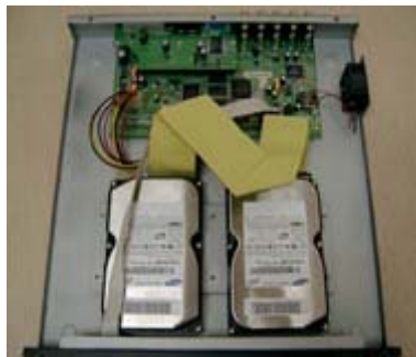
Two HDD Installation
