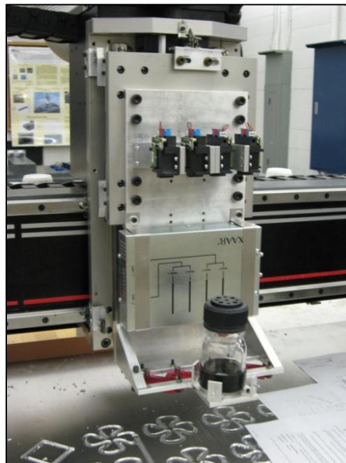
Figure 18 Carriage assembly mounted on Z-axis
