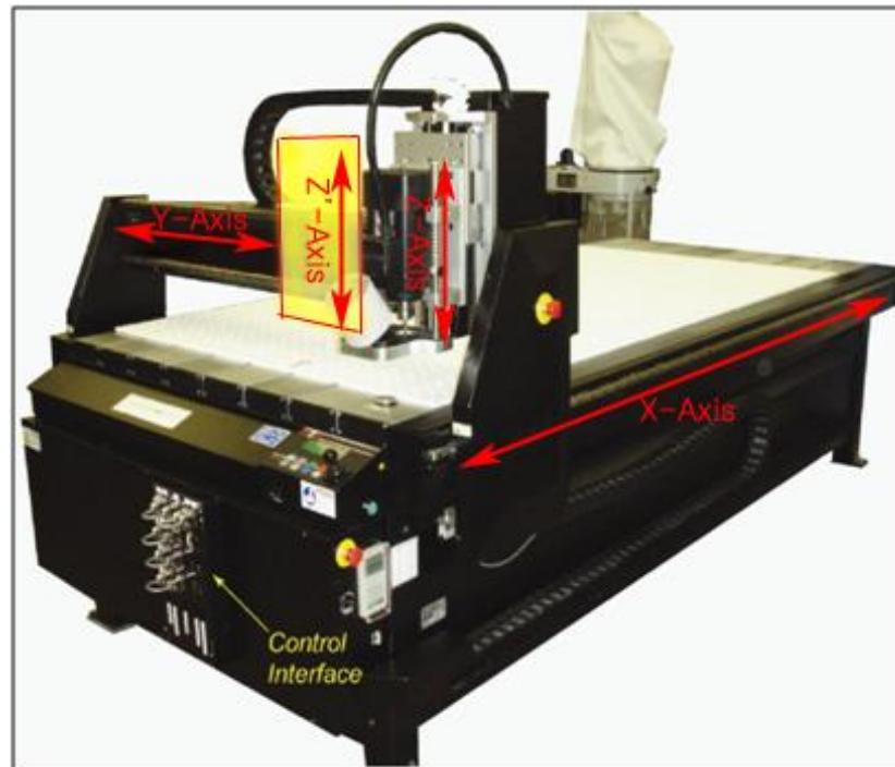
Figure 3 Z'-Axis drive installation location plan
