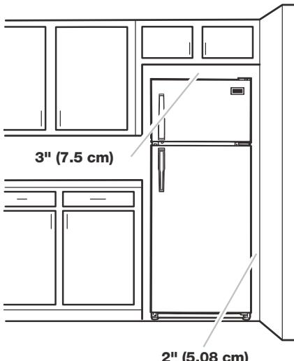
To ensure proper ventilation for your refrigerator, allow for a 1/2" (12.7 mm) space on each side. Allow 3" (7.5 cm) of space between overhead cabinets and refrigerator top. Allow at least 1" (25.40 mm) between back of cabinet and the wall. If your refrigerator has an ice maker, make sure you leave some extra space at the back for the water line connections.
