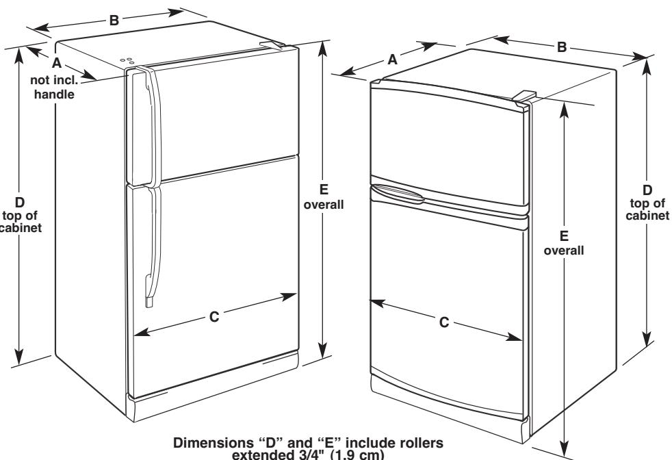
Dimensions "D" and "E" include rollers extended 3/4" (1.9 cm)
