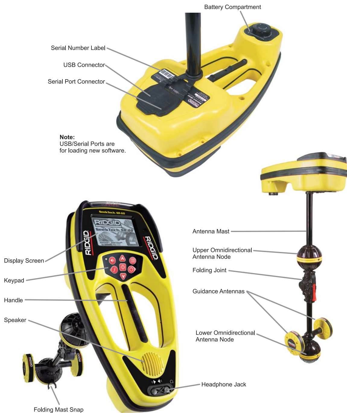
Figure 1: SR-60 Components
