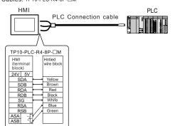
User-made cable is necessary, depending on the PLC. For the detail, refer to TP10 Series Connection Manual.
