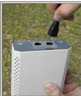
**Step 4** Run the crossover Ethernet cable from Data Input Port (on the front of the PoE Power Injector) to the Ethernet Port on the PC or notebook.
