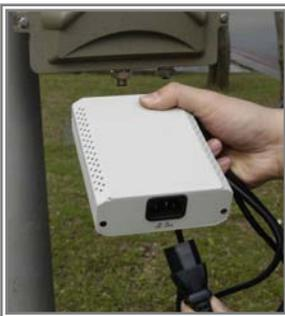
**Step 3** Plug the RJ-45 Ethernet connector, which is from Aphelion 500AG, into the Power & Data Output Port on the front of the PoE Power Injector, when the Access Point receives power over the Ethernet cable, the Access Point will start its boot sequence and the Active LED on the front of the PoE will light up.
