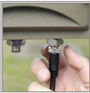
**Step 6:** Attach the RS-232 Cable (Console Port cable) to the Serial Port. Attach the other cable end (with a marked black spot) to the Serial Port on a PC for setting up initial configuration information; another cable end for antenna alignment /deployment tools.
