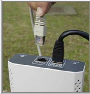
**Step 5** Plug the MIL-C-5015 RJ-45 Ethernet cable into the MIL-C-5015 Ethernet port on the back of the access point.
