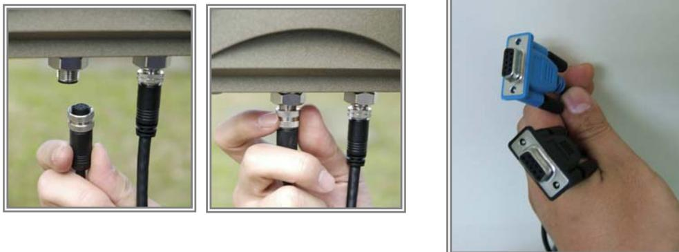
**Step 7** Attach the antenna to the antenna connector as shown in following figure.
