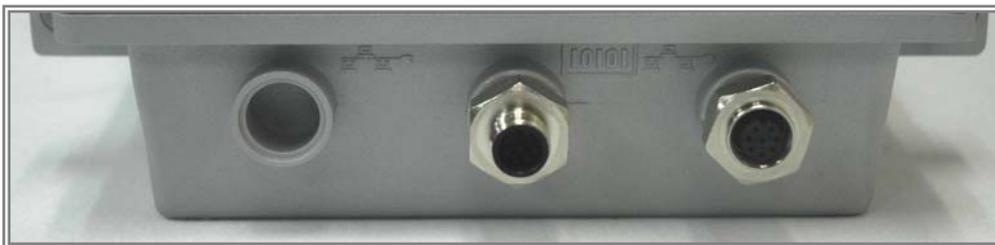
**Power / Signal connector port** : 8-pin female connector with MIL-C-5015 IP67 water proof Connecting to the indoor interface unit supplying the power and signal.
