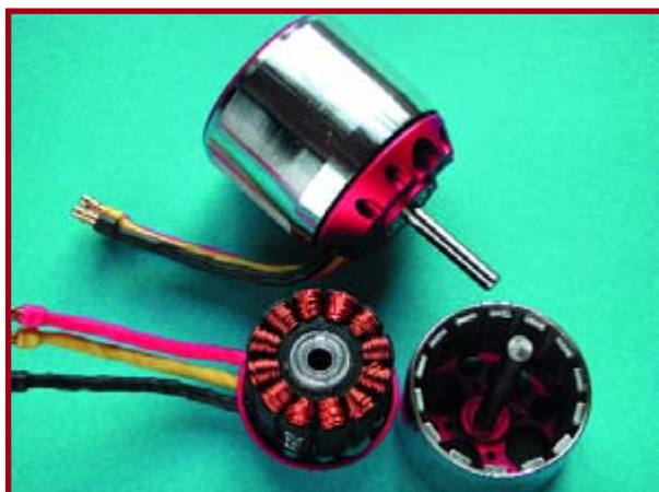
Figure 14. Brushless motor with exterior rotor designed for use in models.
