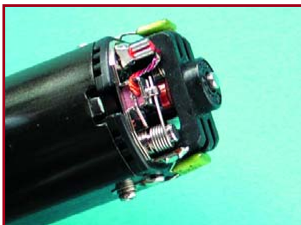
Figure 5. The brush system in a mechanically-commu- tated DC motor is com- plex, lossy and prone to wear.
