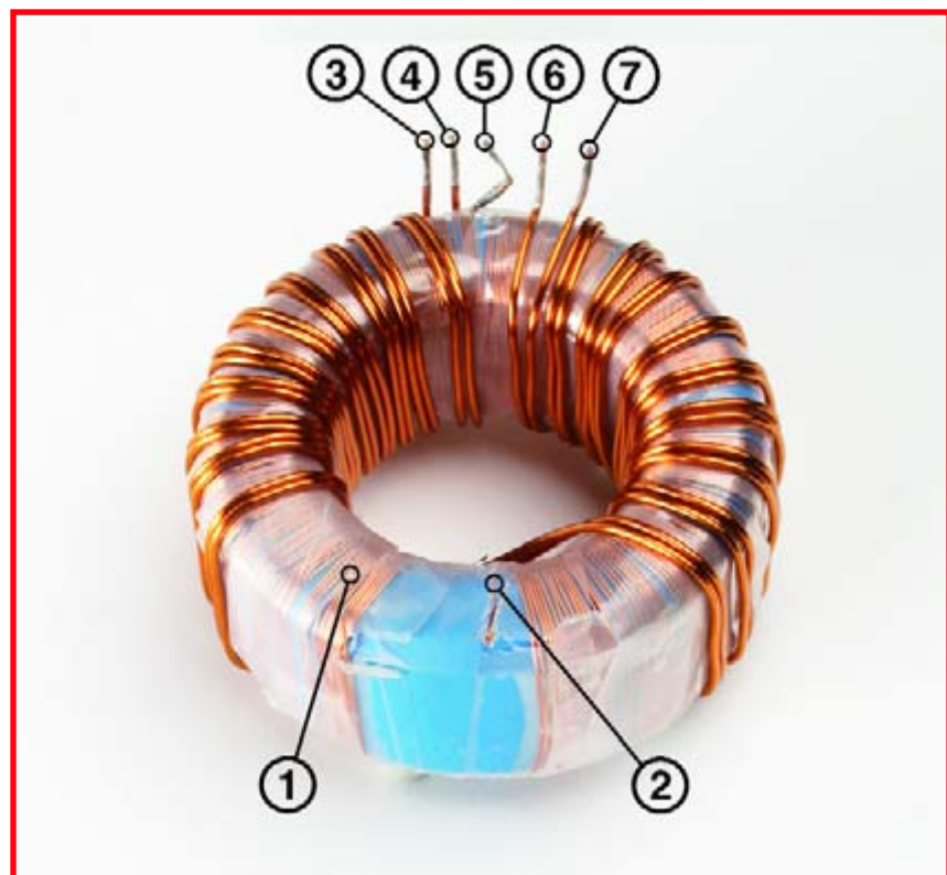
Figure 8. This shows how you should wind the transformer. Although this is version 2.0 of the transformer (as opposed to version 3.0 in the photo of the prototype), the winding method is the same. Legend: ① = C4 in the schematic; ② = C1; ③ = B2; ④ = A2; ⑤ = C2 and C3; ⑥ = B1; ⑦ = A1.
