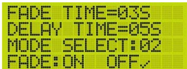
Press ◀ or ▶ to shift FADE TIME, DELAY TIME, MODE SELECT and FADE ON/OFF.
