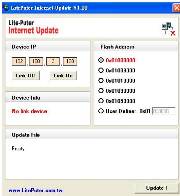
STEP4 : Set the IP address on Device IP setting, after setting press Link On.
