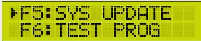
STEP1 : Press ▲ or ▼ to select F5, then press **ENT** and LCD will display,
