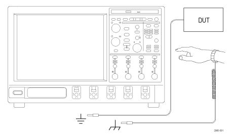
**2.** Discharge the static voltage from all cables before connecting them to the instrument or to the device under test (DUT). Before you attach the cable to the instrument, you can momentarily ground the center conductor of the
