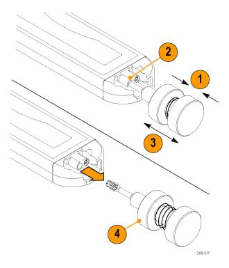
**Install Bullets.** When both bullets have been removed, install new bullets. To do so, follow these steps:
