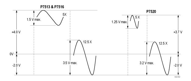
**Offset Voltage Range.** Offset voltage ranges are as follows:
