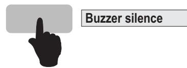
**2** Silence the alarm devices by pressing the "SILENCE/RE-SOUND" - button
