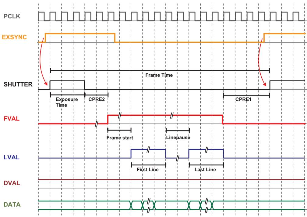
Figure 5.10: Timing diagram for external trigger mode
