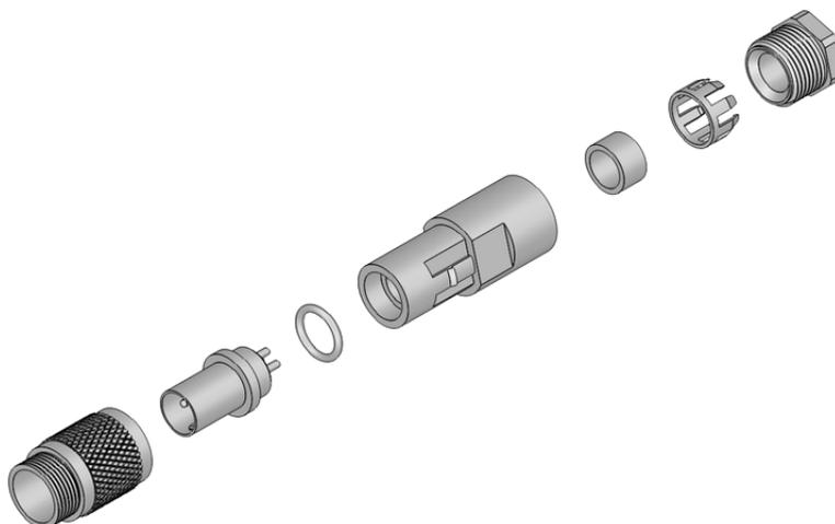
Figure A.1: Power connector assembly
