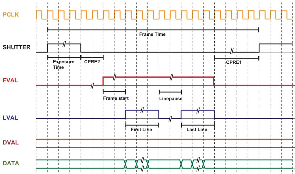
Figure 5.9: Timing diagram for free running mode
