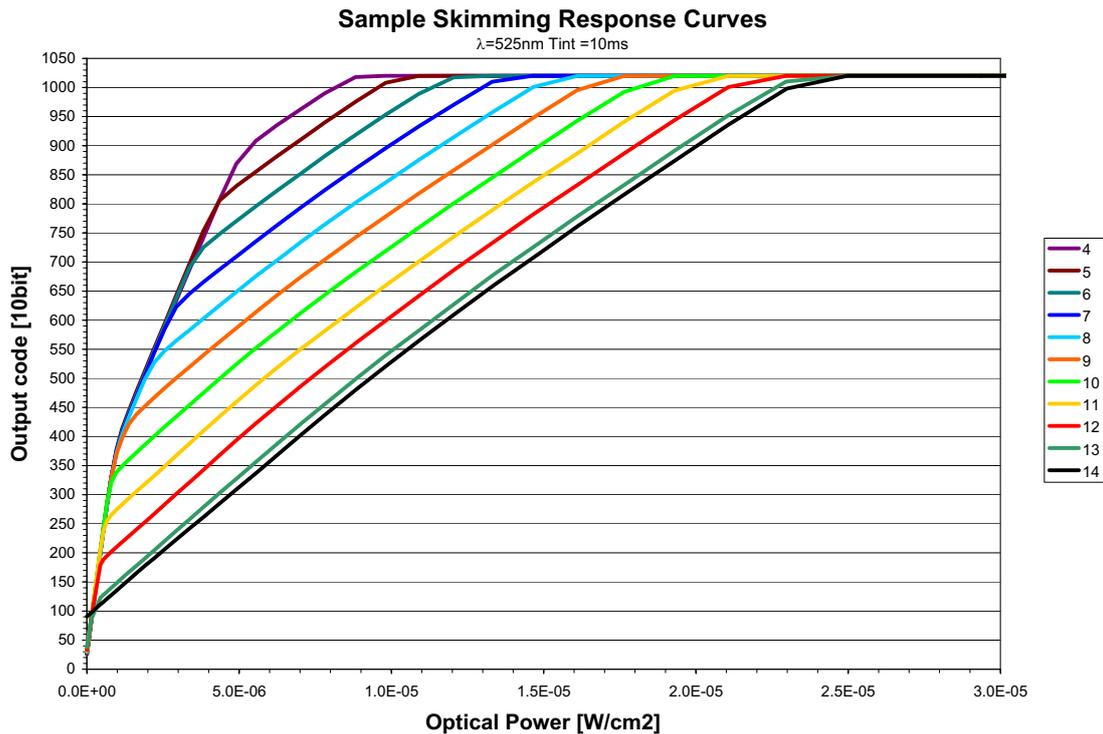
Figure 4.6: Response curve for different skim settings
