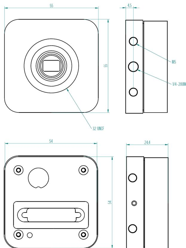
Figure 7.1: Mechanical dimensions of the BLIZZARD-60 model with CameraLink interface
