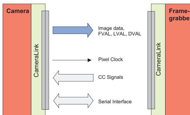
Figure 4.8: CameraLink serial interface for camera communication
