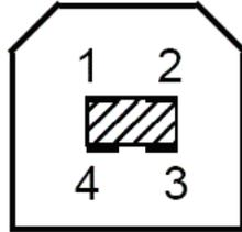
Figure A.5: USB type B connector (front view)
