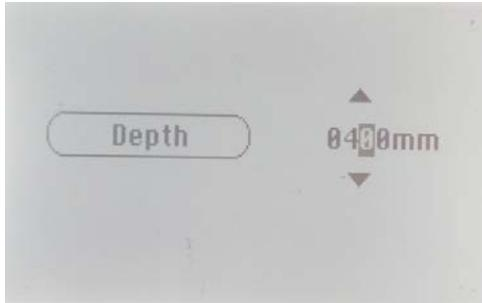
Figure16 Display, the decimal to be changed is highlighted.
