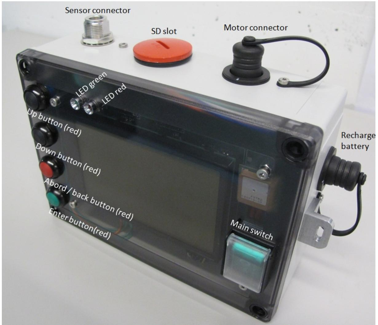
Figure2 The new controller of the SnowMicroPen 3.
