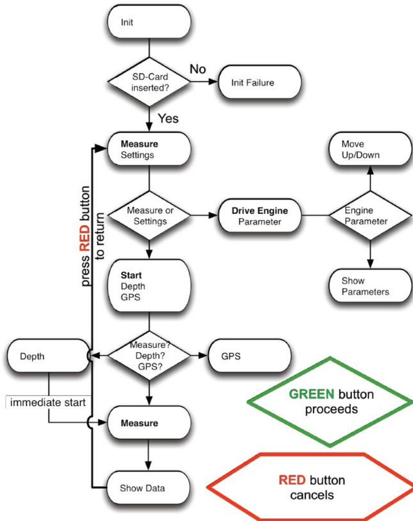
Figure5 Flowchart of the menu structure.
