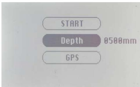
Figure14 Display to change the default measure length [mm].
