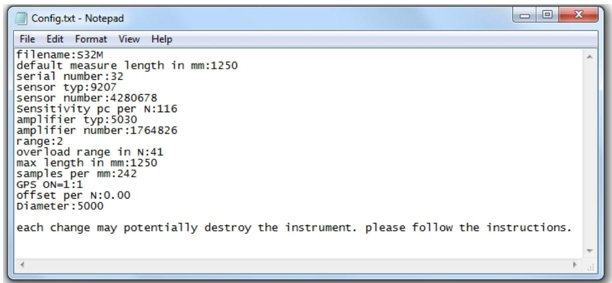
figure4 Example of a configuration file that must be stored on the SD-card.
