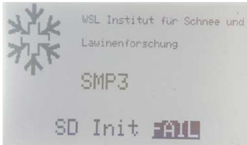
Figure6 Display if the initializing of the SD-card fails.
