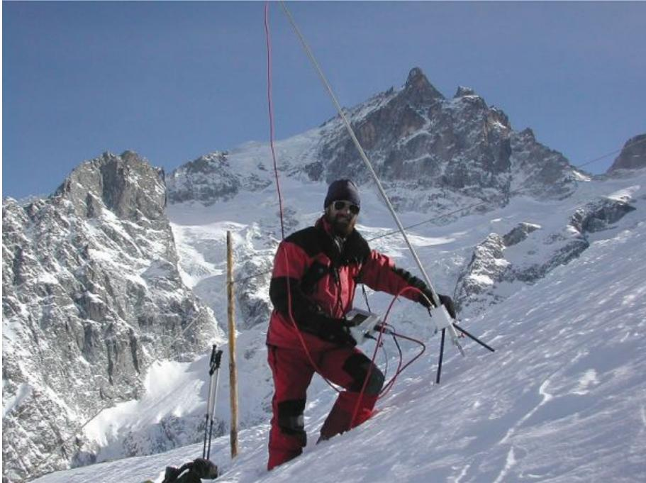
Figure1 The SnowMicroPen must be positioned perpendicular to the slope.
