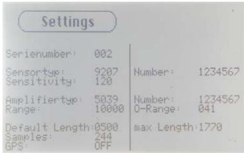
Figure9 Display shows settings from configuration file on the SD-card.
