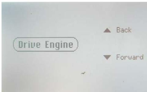
figure 10 Display to drive the SMP manually.
