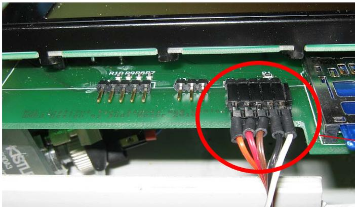
3. Five-pin plug on the left side of the SD-card. **White wire on the right side of the plug**
