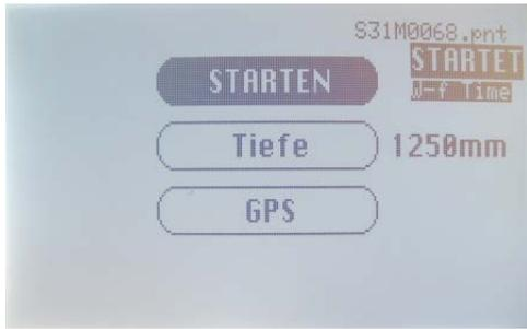
figure 12 Display of initializing the measurement after pressing the green button for the first time. The display shows the message "W-f-Time", means wait for time of the GPS signal. This W-f-Time process can be jumped over by pressing the green button for a second time.
