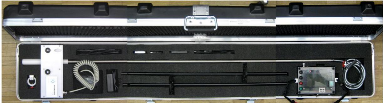
Figure17 Box for transportation of SnowMicroPen 3 containing all components.
