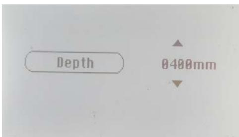
Figure15 Display in the menu for changing the measure length [mm].
