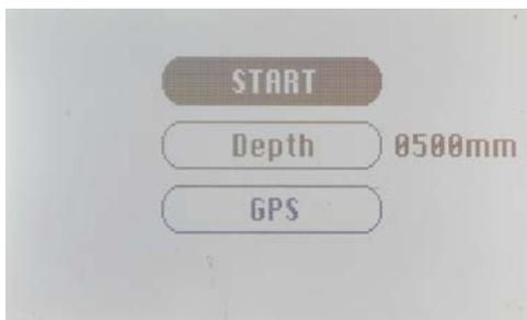
Figure11 Display to start a measurement with the default length of 500 mm, change the default length (depth) or settings of the GPS (optional - not included in standard version of SnowMicroPen).
