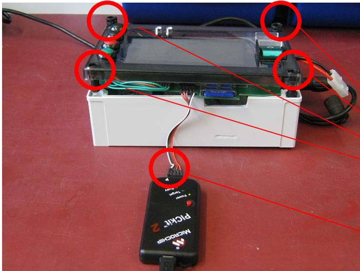
1. Loosen the four screws of the SMP controller cover
