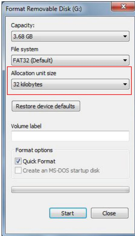
figure 3 Parameter to reformat the SD-card.
