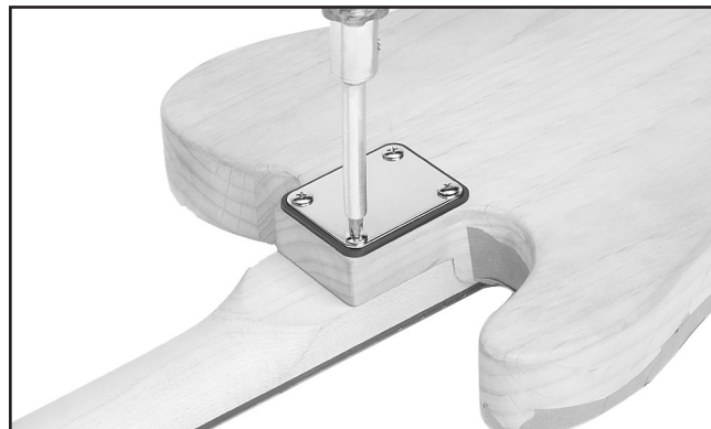
Figure 10. Fastening neck to body.
