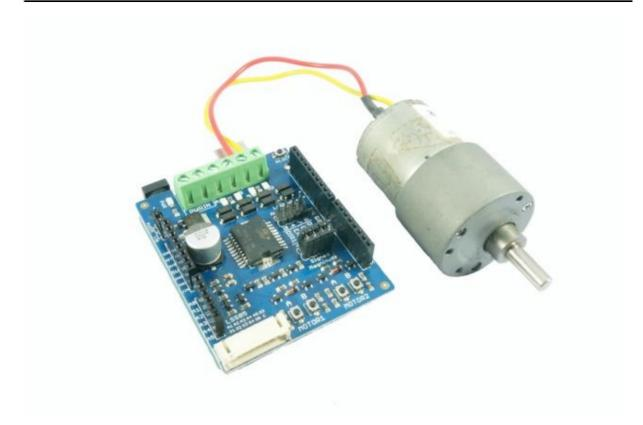
Connect motor to the MOTOR1 and MOTOR2 terminal block. Upload SHIELD-2AMOTOR example code to Arduino. Or you can test directly by using test switch.
