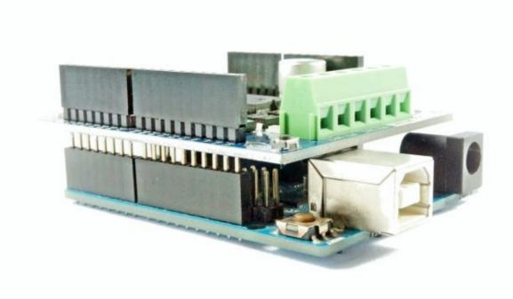
Figure above shows that SHIELD-2AMOTOR is stacked on the Arduino UNO.
