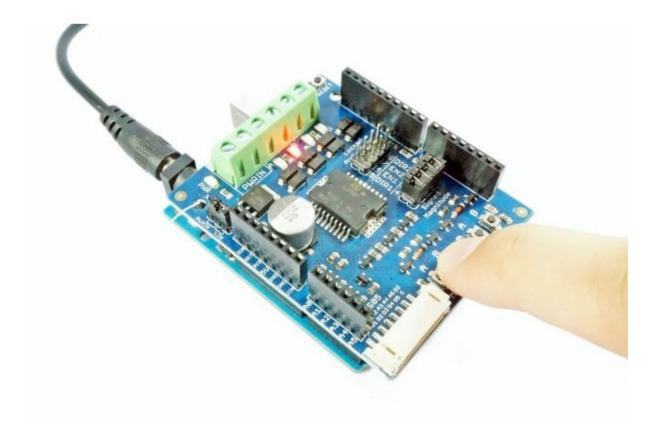
SHIELD-2AMOTOR also include with <u>LSS05</u> connector. Means you can plug in LSS05 directly to Arduino.
