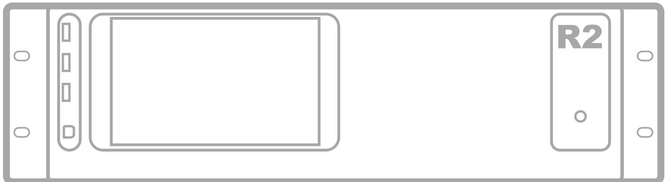
On the front of the R2 amplifier are a power button, four USB connection ports space for an optional touchscreen (R2DIS) provided.
