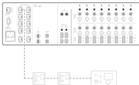
Multiple DW3018/4018 and one DW5065 Wall panel on one PI Port (PI1 to PI8)
