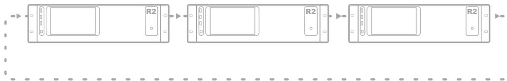
To control all the functions of all the R2's in one network, only one connection with the ethernet network of one R2 in the ring network is required. When multiple R2's are connected in a ring network, first a selection box will be displayed whereby can be selected which R2 you want to control.
