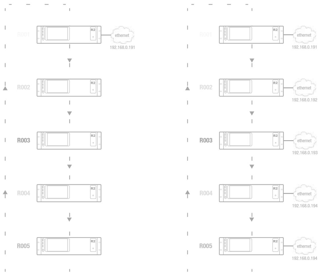
Example setup with 5 R2's, on the left side with only one Ethernet connection (Method 1) while on the right side every R2 has a separate ethernet connection (Method 2)
