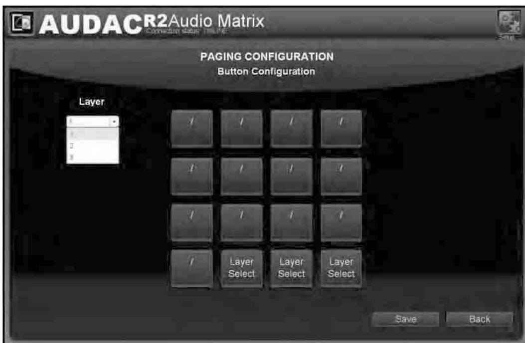
After this button is clicked, a windows comes up allowing you to select the function which should be performed after pressing this button. The available functions shown in the dropdown list on the left side are "Zone Select" and "Play Message".
