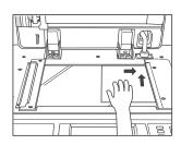
Be sure to select the desired original set direction by selecting SPECIAL ORIGINAL on the Basic Screen and selecting the original set direction. Touch OK.
