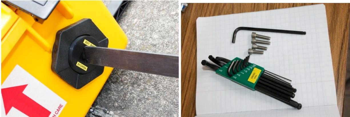
**Fig. 9:** Hand tools required are: possibly a tool for a 2x2 cm female square for the air caps if you can't do it by hand (left), imperial hexagonal or Allen keys (left)
