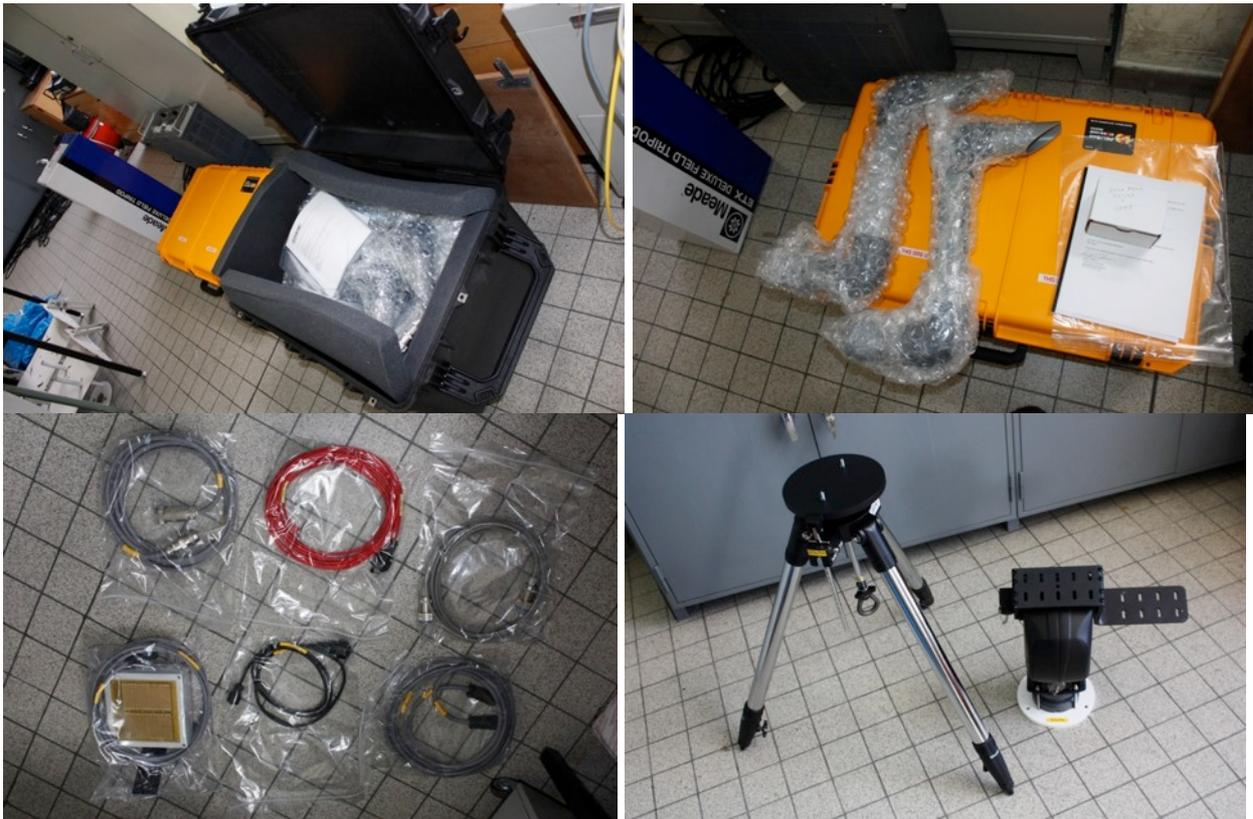
**Fig. 7: SAM parts: all 3 boxes with the black case for the components to mount on foreground (top left), air pipes and manual on the orange control console case (top right) Wires and rain sensor (bottom left), MEADE tripod and FLIR tracking head (bottom right). The instrument head is not shown here (white rectangular box), see the manual or other photos in this document.**
