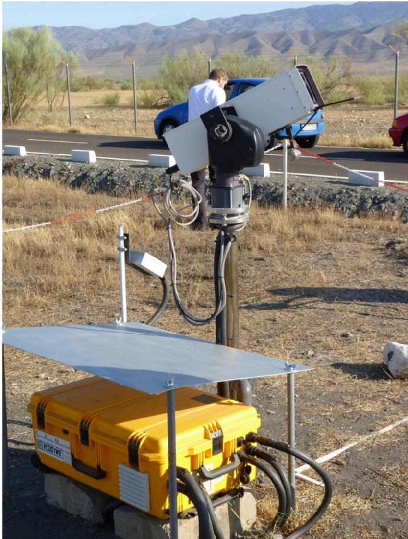
**Fig. 11: DLR SAM system at PSA, with hardware upgrades for long term operation: a removable roof reduces the box temperatures and a custom ground fixed pole has been built for the tracking head. The rain sensor (left behind) is on the original provided pole and 45° fixation. Air venting is done with the white filters instead of the air pipes as on CNRS unit.**
