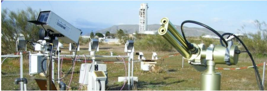
**Fig. 1: Photo of the SAM Series 400 next to the Cimel sun photometer at DLR's meteorological station at the Plataforma Solar de Almería (PSA).**
