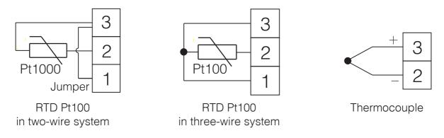
Fig. 4. Connection of input signals
