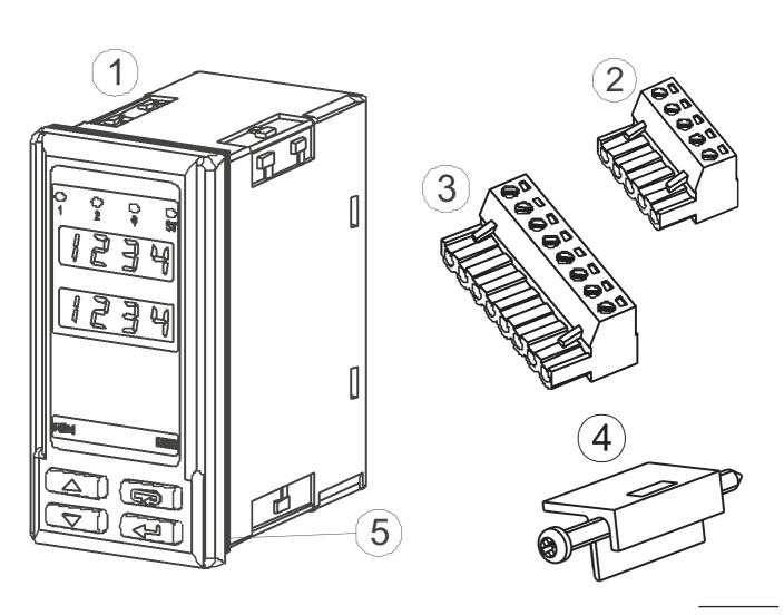
The delivered controller set is composed of:
