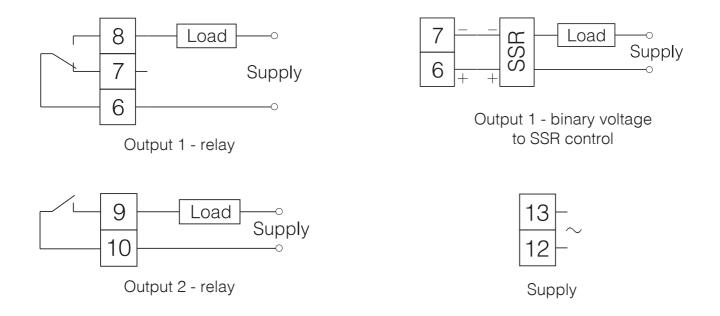
Fig. 5. Supply and load circuit connection
