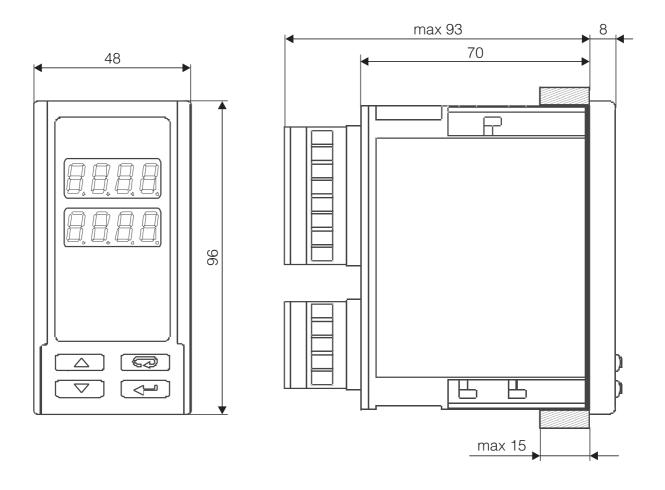
Fig. 2. Controller overall dimensions
