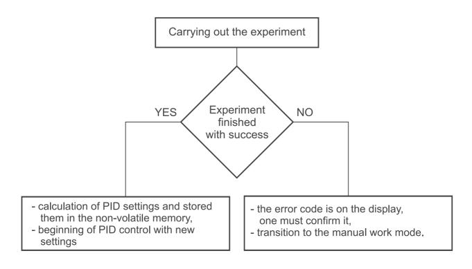
The auto-tuning process will be broken without PID settings calculation, if a controller supply decay occurs or the button is pressed. In such a case, the control with current PID settings will begin.
