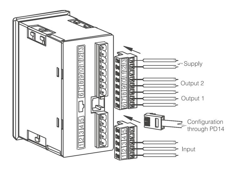
Fig. 3. View of controller connection strips
