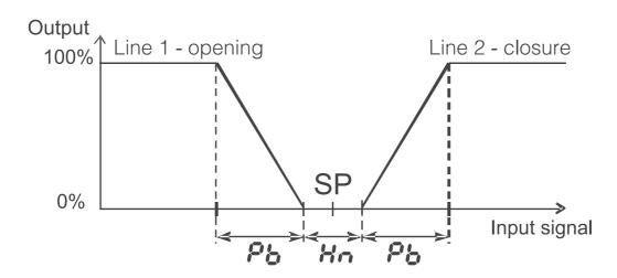
Fig. 11. Step-by-step three-state control
