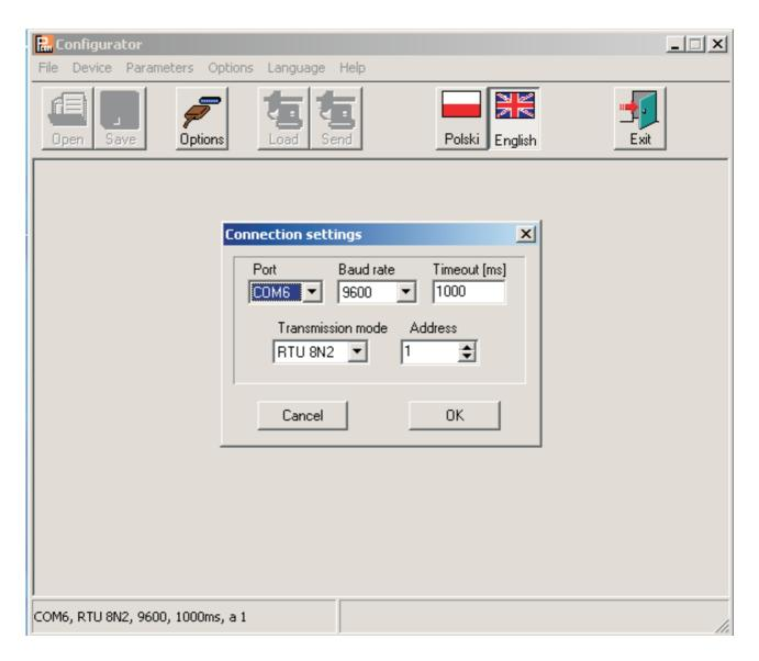
Fig. 13. Connection configuration to the RE81 controller.
