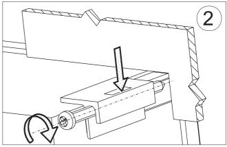
Fig. 1. Controller fixing in the panel.
