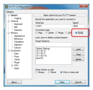
Configure the serial port correctly (see image below). Click Open and power on the rBOX630.
