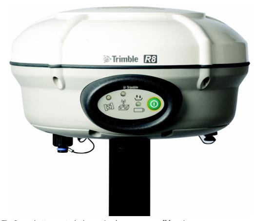
The Power button controls the receiver's power on or off functions.
