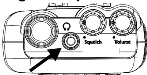
For private listening, you can plug a 3.5 mm mini-plug earphone or mono headphones (not supplied) into the headphone jack on top of your scanner. This automatically disconnects the internal speaker.
