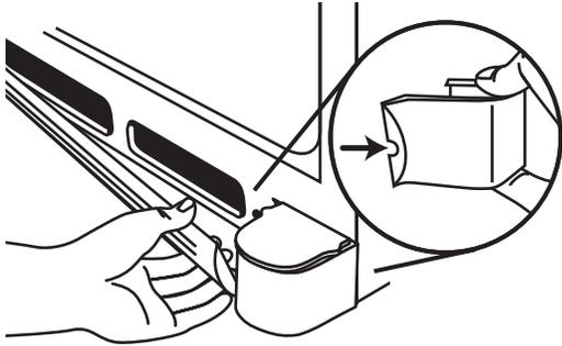
3. Using a screwdriver or  $\frac{3}{8}$ " hex driver, turn the roller adjustment screw on each side to raise or lower that side of the refrigerator.
