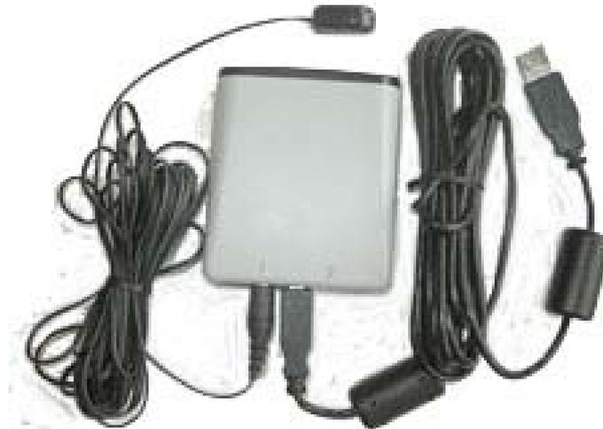
Media Center remote controller infra-red receiver box and infra-red receiver for set top box remote control function
