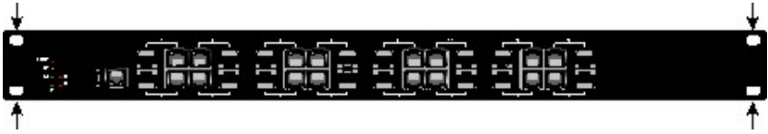
Figure 9: Mounting in the switch cabinet
