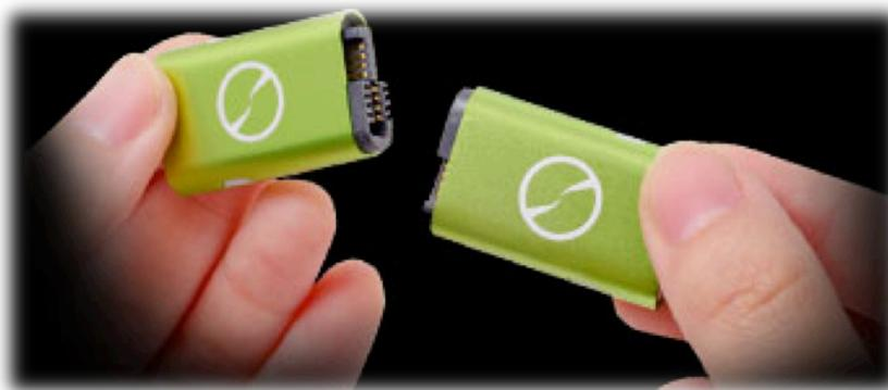
8. If you intend to use iTwin only for SecureBox and not for Remote File Access, then unplug the paired iTwin device and separate the two halves. These two halves will now act as your iTwin SecureBox keys. We suggest keeping one key in a safe place. Carry the other key with you.
