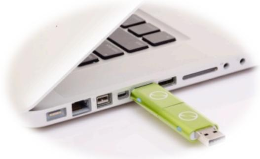
1. Join together the two halves of your iTwin device, to form a pair, and then insert the paired device into a USB port on your computer. Open your Finder window. In 'Devices', click the 'iTwin' CD-ROM device.
