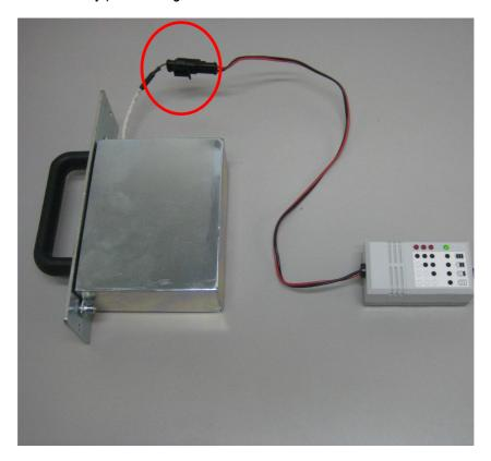
6) Insert the power supply (12Vdc) to the power outlet at 230Vac and connect it to the charger through the jack.
