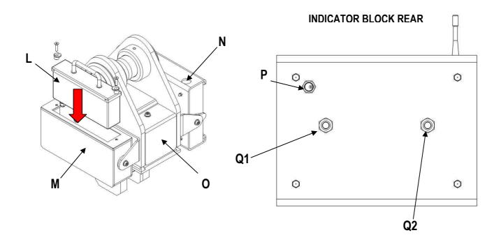
L: is the battery box and its direction of insertion into the MCWHU electronic crane scale;
