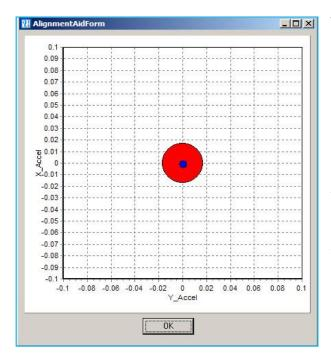
This will bring up the screen opposite. The blue dot is the position of the IMU with respect to both the X and Y axis and the red circle is a target area for the blue dot.
