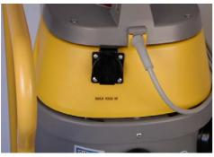
hand tools direct to the power outlet of the motor top, the RONDA<sup>®</sup> 1200H / 1200H-S will automatically be switched on and off, when the hand tools are switched on and off.
