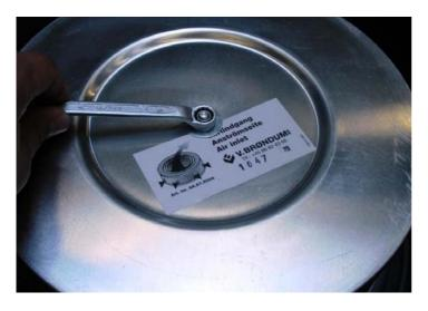
Loosen the HEPA-filter. Use a ring spanner size 10.
