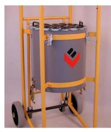
The large multi-tube filter of the RONDA<sup>®</sup> 1200H / 1200H-S is mounted in the filter container. The multi-tube filter has been tested with quartz-dust particles, of which more than half is less than 5  $\mu$ m (5  $\mu$ m is the same as 0.005 mm). The filter holds back 99.97% of all the particles, which corresponds to an emission of 0.06 mg/m<sup>3</sup> in the purified air.
