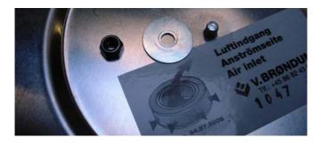
Mount the washer and the nut. Tighten with approx. 25 Nm.
