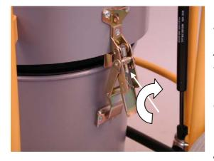
The container clips ensure that the collection container is held up against the filter container.
