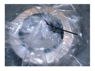
Close the bag with a cable tie. Dispose of the filter according to the national regulations.
