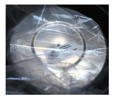
Pull a plastic bag (100  $\mu m$  or the like) over the used filter.
