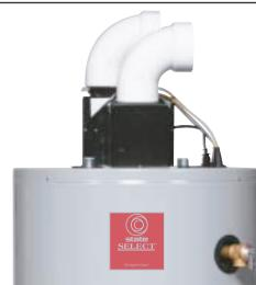
**Power Direct-Vent Design** – Two-pipe closed-combustion system draws all make-up air from outside the home, eliminating problems caused by insufficient indoor ventilation. For installation versatility, system permits combined horizontal and vertical venting and air intake runs up to 45 feet (including one 90° elbow) using 3" Schedule 40 PVC, CPVC or ABS pipe.
