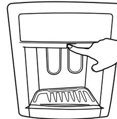
The faucet rotates to the center automatically. However, you must rotate it back into place manually. When in place, it will click.
