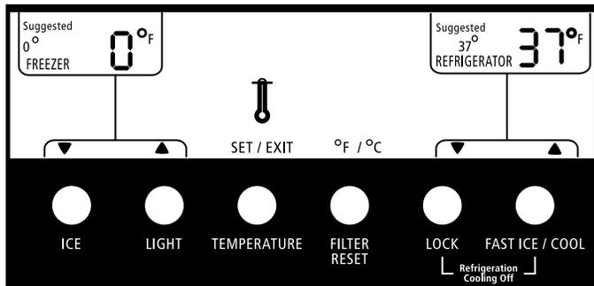
**NOTE:** To view Celsius temperatures, press the FILTER button when adjust mode is activated. To return the display setting to Fahrenheit, press FILTER again.
