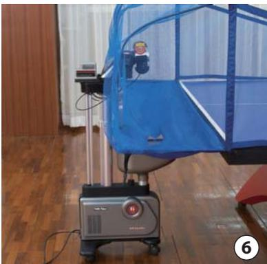
6. Always unlock the robot wheels before moving the robot. Roll the robot to the table.
