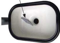
The capacity of the Ball Container is 100, 40mm balls. The container should not be filled above the yellow line inside the container. Anything other than table tennis balls in the Ball Container may damage parts and adversely affect the robot's normal operation.
