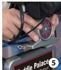
5. Insert the Spin Indicator Panel into the slot of the net. If you need to disassemble the net, remove the Spin Indicator Panel first.
