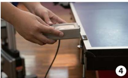
4. Clamp the LCD Panel support to the edge of the table and insert the Touchscreen LCD Panel into the support. Remove the protective film before operating the panel.
