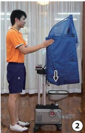
2. Partially unfold the ball collection net and carefully slip it over the robot head. Insert the double pin into the net support connector, located on the robot frame.
