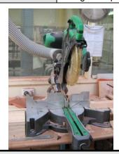
**Potential Hazards:** Exposed moving parts and electrical hazard with the potential to cause harm through entanglement, impact and cutting, exposure to noise, dust, projectiles and sharp objects.
