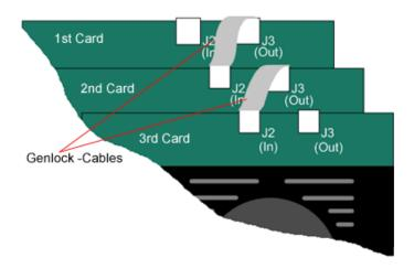
Continue to connect the genlock cables J<sub>3</sub> (Out) to J<sub>2</sub> (In) until all cards are connected.
