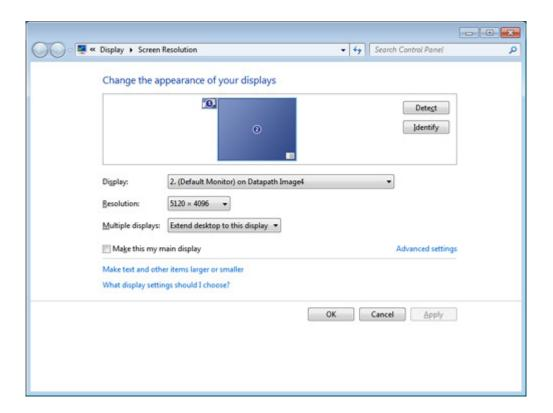
If you have more than one graphics device in your machine, the Display Settings allow you to control which graphics devices are used and what their position on the desktop is. There should be a monitor icon for each ImageDP4 card and at least one monitor icon for each of the other graphics devices in the system (there is a limit to the number of monitor icons that are displayed).
