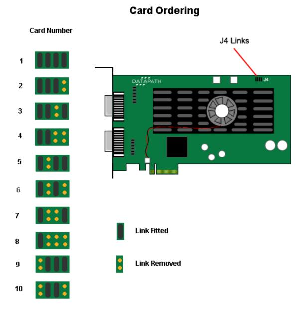
The links control the order in which the display driver uses the ImageDP4 cards. Knowing the order in which the ImageDP4 cards are used is useful when connecting the screens and the outputs from video switches.
