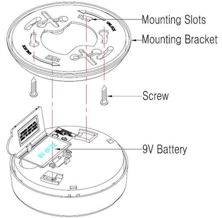
1. From back of heat alarm, remove the mounting plate by turning it counterclockwise.
