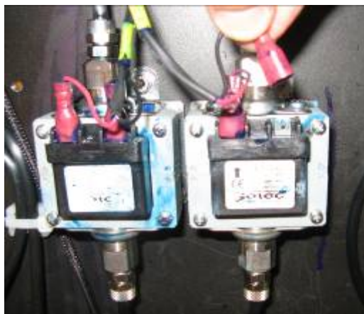
Figure 3: Disconnecting the old AC Pump
