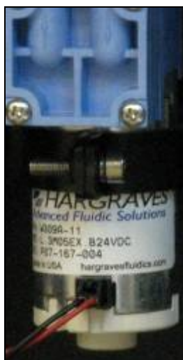
Figure 4: Disconnecting the new DC Pump
